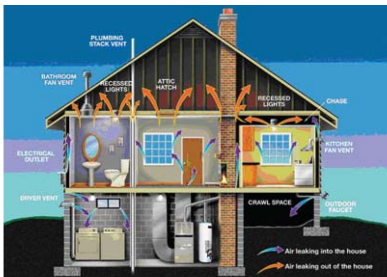
Plug that leak! This diagram shows typical air movement within a house.
